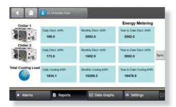
Trane **EnerView** meters the energy consumption of each chiller and calculates the cooling capacity produced by the plant. An on-screen dashboard shows the daily, weekly and yearly consumption and cooling capacity.
